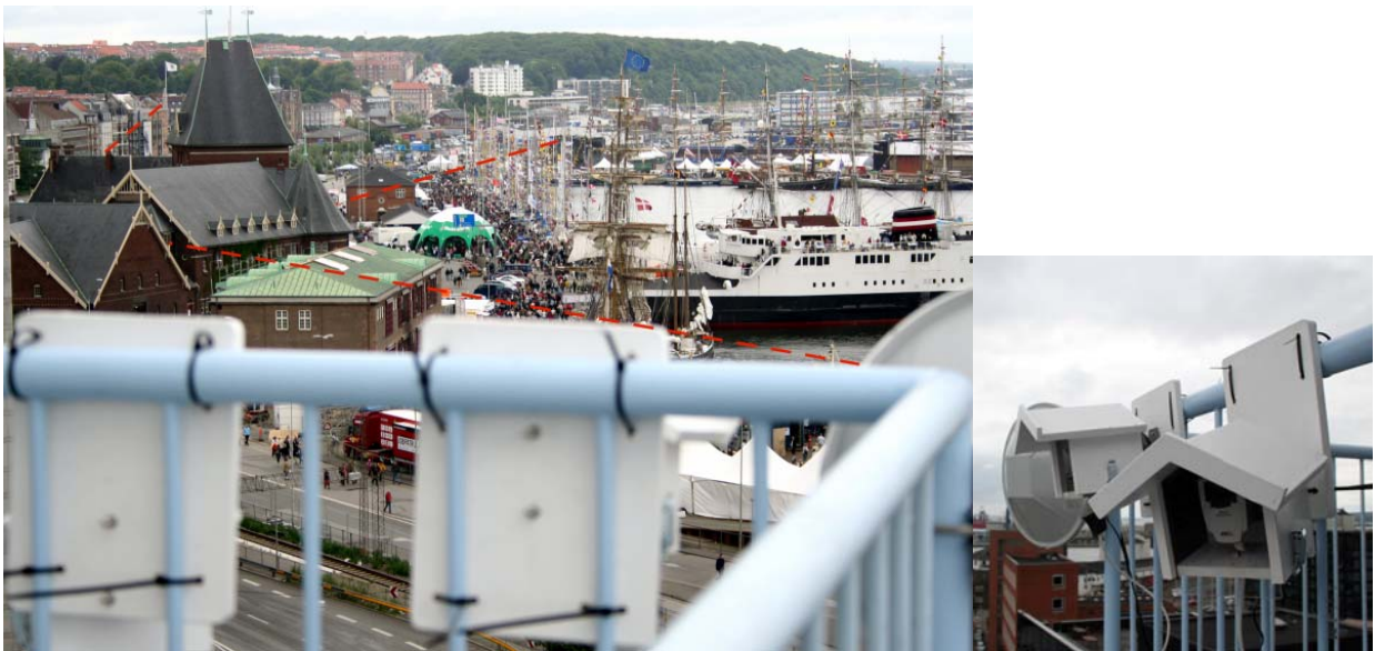
The red dotted lines indicate directional WiFi connections. The white plates in the foreground are the back of two cameras and a disk used for directional WiFi.
