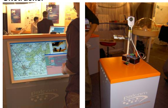
Figure 2: Left: The dotted lines on the map show the angle of view "seen" by the sitetracker. The picture in the upper right corner shows the picture from the webcam. The diagram in the lower right corner shows the palcom architecture (service browser). Right: The webcam with compass and motor.
